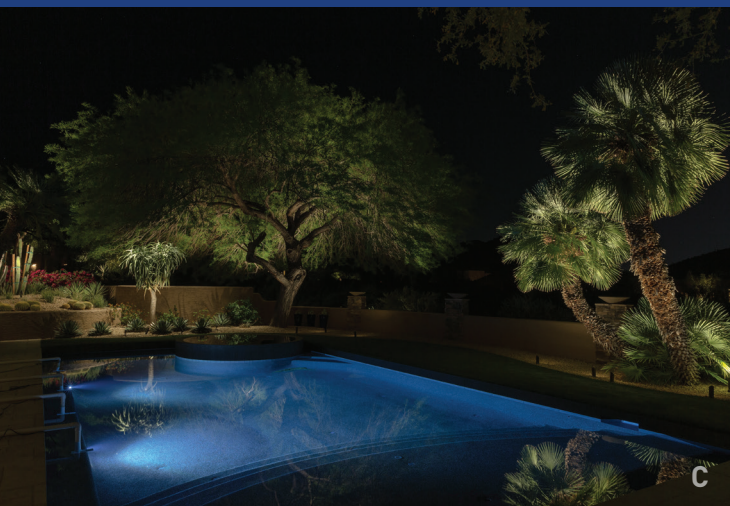
Photo B above features the same scene with standard non-dimmed 15-watt pool lights (too bright) set to deep blue, 12-foot spacing (too wide). Photo C below features the same scene with standard non-dimmed 15-watt white pool lights with 12-foot spacing. Note: This is a dark interior pool, Pebble Sheen Turtle Bay. A light interior pool will MOST DEFINITELY benefit from dimmable lights.
